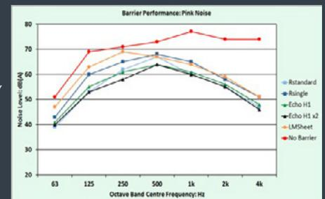
• Attenuation at 10m - - "A" weighted noise levels - High frequency diamond drill noise source
