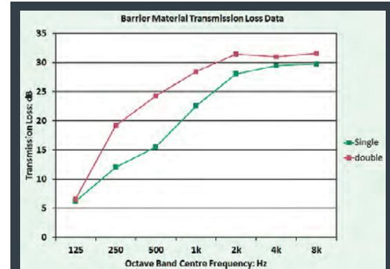
**Barrier Material Transmission Loss Field Data - dB**
